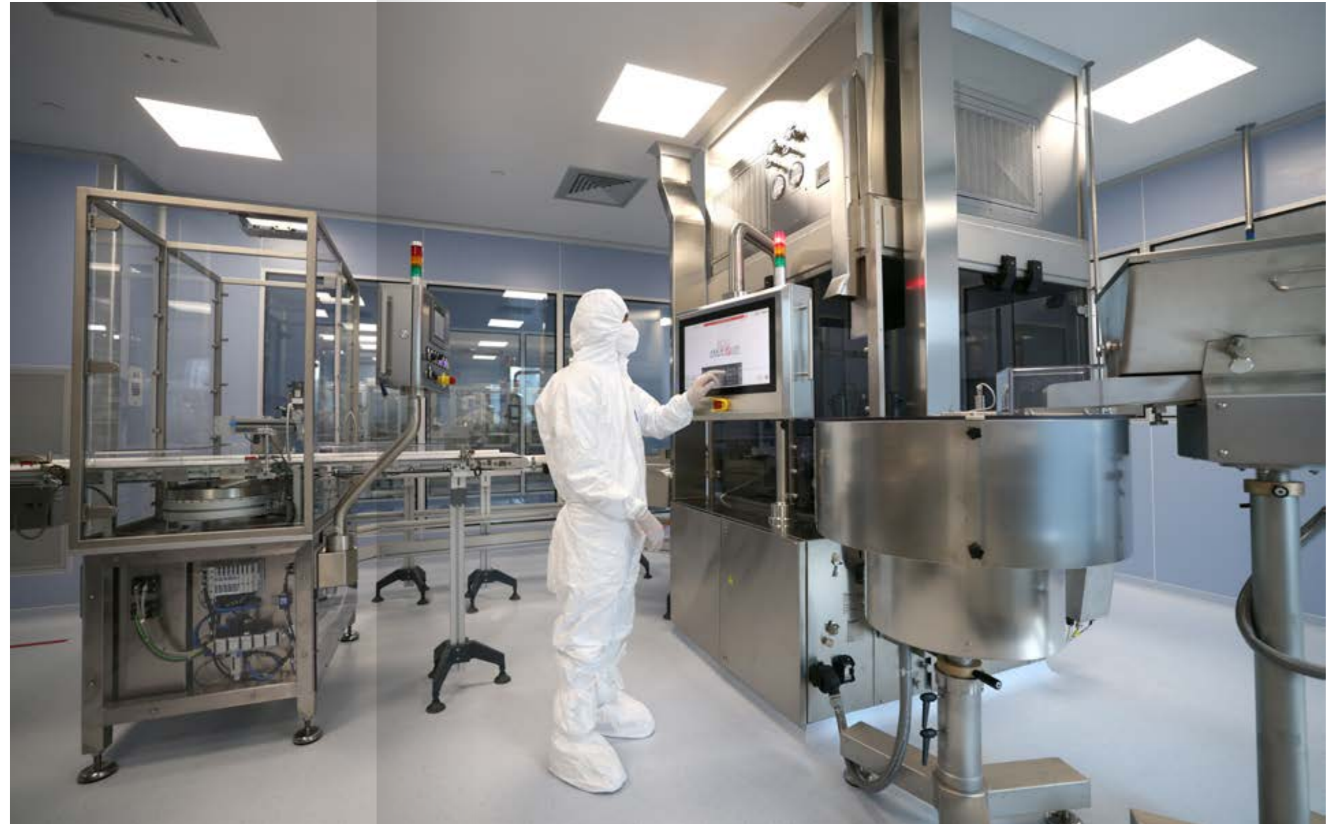
Digital control and monitoring of the production line via touchscreen
