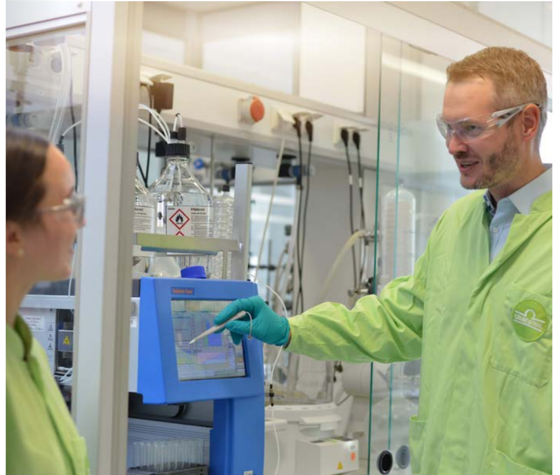
Grünenthal employees in the chemistry laboratory in front of a flash chromatography device
